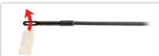
1. Place a few drops of silicone oil or teflon oil on the cleaning cloth and wind around the rod.
