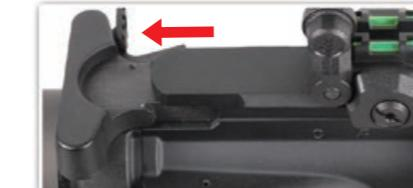
Pulling the charging handle will take the bolt back and open the port cover.
