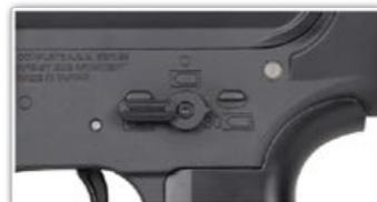
3. When you've confirmed the Setting Menu you want to enter, switch to AUTO to enter Setting Mode. In Setting Mode, every trigger pull cycles the different Mode options in descending order, as seen on the list on the right.
